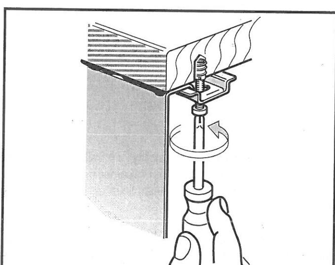
4. Tighten the brackets and remove any excess sealant.
